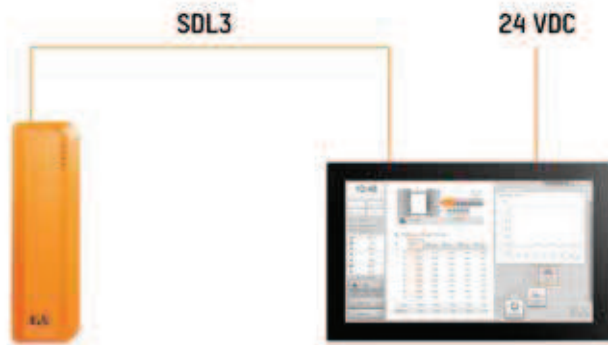
If 24 VDC is already being supplied, the Automation Panel can be connected directly to the Automation PC 910 via SDL3.
